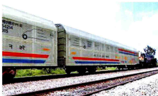
BCACBM rake used for vehicle transportation
